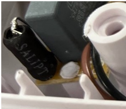
Figure 5: PCB held in place via melted plastic
