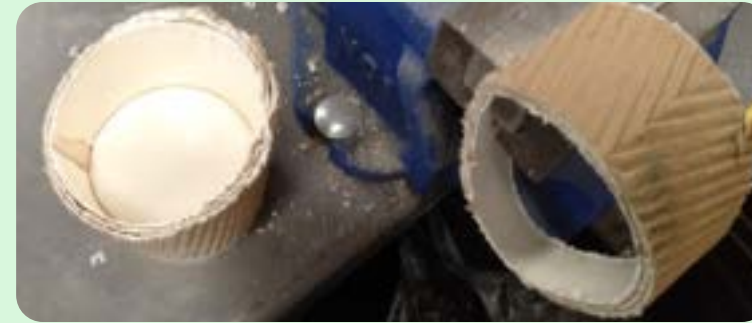
Detach the base to get the cup ring.
