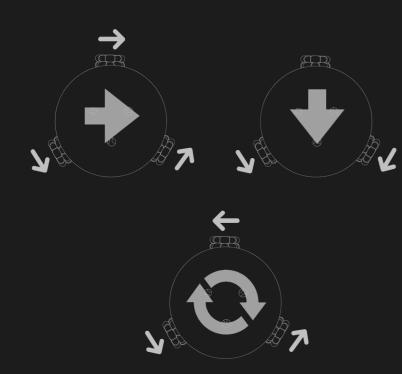
Gizmo Bot is an omnidirectional robot allowing for movement in all directions with ease with just three omniwheels. This makes it ideal for programmed sequences as it can fit within tight spaces and has a high level of manoeuvrability.
