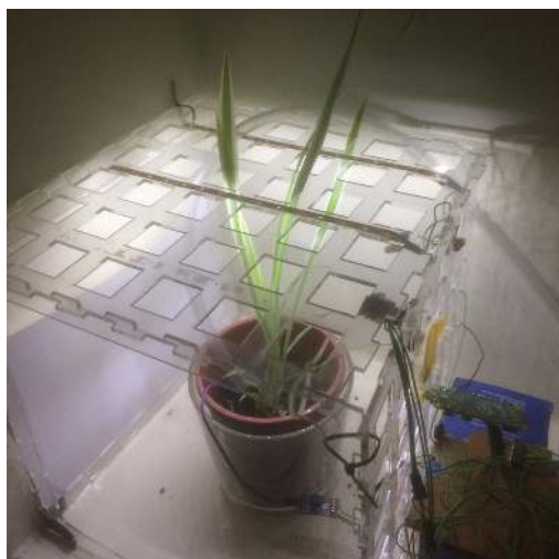
A prototype self-regulating plant system using a Raspberry Pi computer (would be replaced by a PLC)
